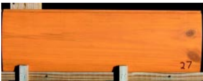
Lifeline Ultra-2, After accelerated weathering
