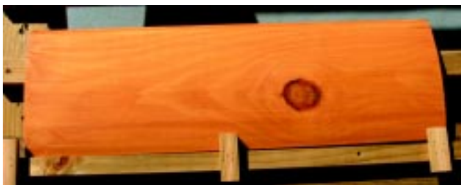
Lifeline Ultra-1, Start of accelerated weathering
