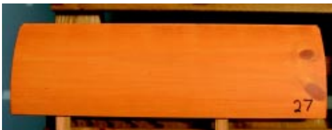
Lifeline Ultra-2, Start of accelerated weathering
