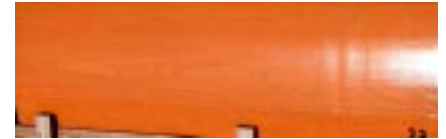
Panel with Dark Honey stain, Lifeline Advance Gloss topcoat. Exposed to accelerated weathering conditions and harsh winds, dirt and sun for one year.
