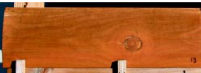
Lifeline Ultra-1, After accelerated weathering
